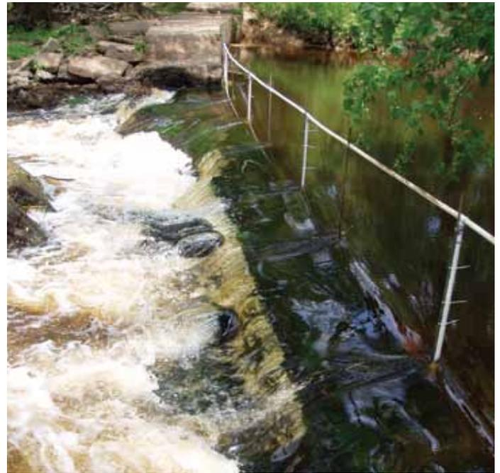
*A PIT antenna located at a notched dam will record movements of tagged fish in the river (Josh Raabe; NC Coop Unit).*
